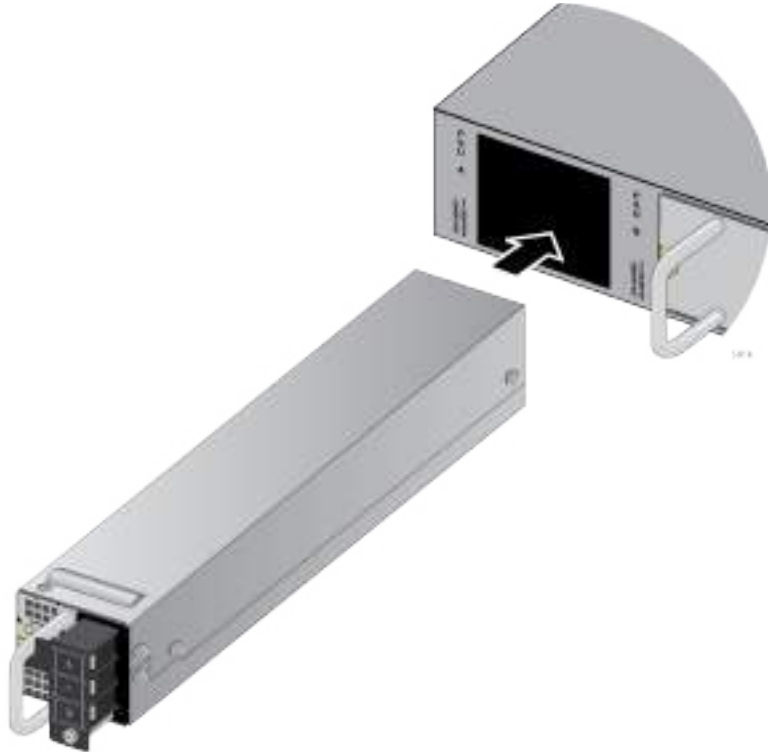
Figure 58. Sliding the PWR600 DC Power Supply into the Chassis
