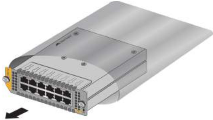
Figure 73. Removing the Ethernet Line Card from the Anti-static Bag
