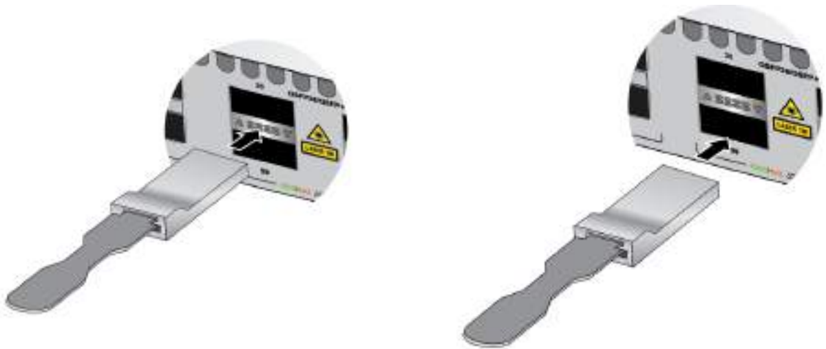
Figure 131. Installing 100Gbps QSFP28 Transceivers in Base Ports 25, 29, 33, 37
