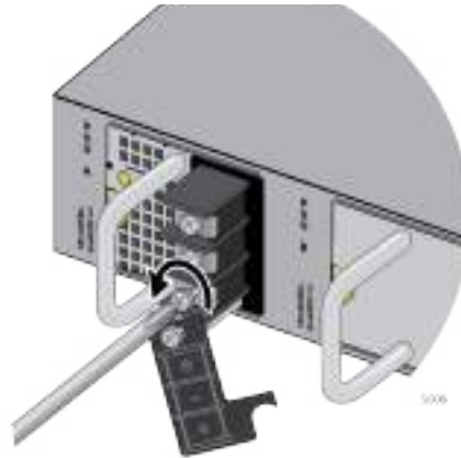
Figure 62. Loosening the Ground Screw
