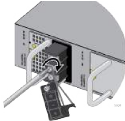
Figure 67. Tightening the Screw for the Negative (-)
