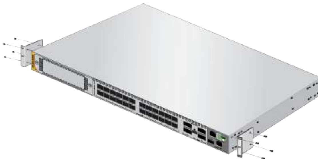
Figure 85. Attaching the Equipment Rack Brackets
