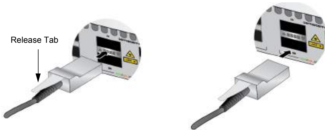
Figure 134. Attaching QSFP+ Cables
