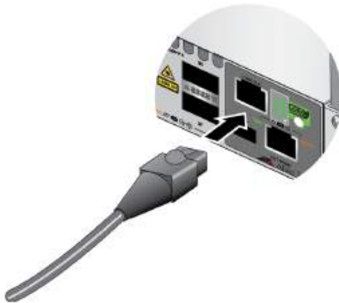
Figure 123. Connecting the Management Cable to the Console RS-232 Port
