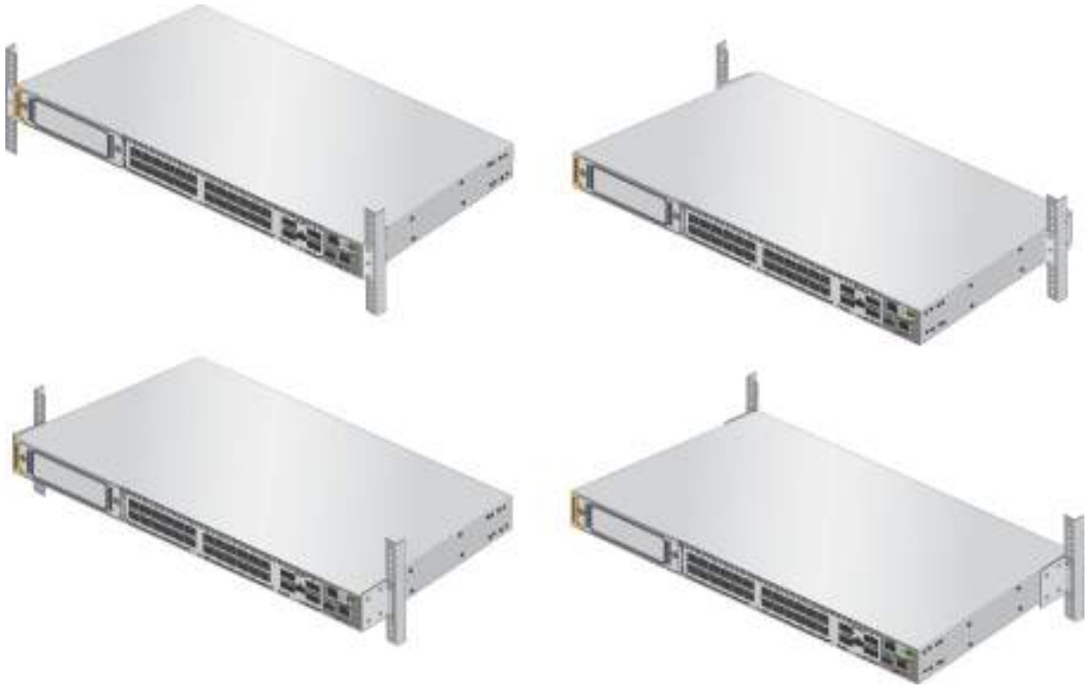
Figure 83. Switch Orientations in an Equipment Rack
