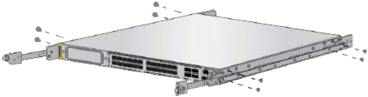
Figure 115. Attaching the Inner Rails to the x950 Switch Go to “Installing the Switch in the Equipment Rack” on page 184.
