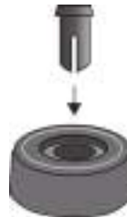
Figure 79. Inserting the Rivet Housing into the Bumper Foot
