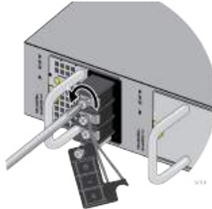
Figure 68. Loosening the Screw for the Negative (+)
