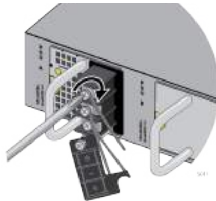
Figure 69. Tightening the Screw for the Negative (+)
