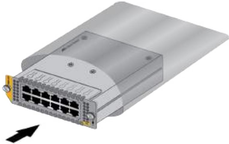
Figure 138. Placing the Ethernet Line Card in its Anti-static Bag
