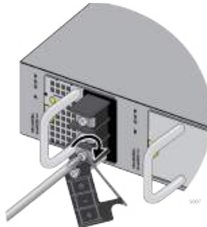
Figure 63. Wrapping the Grounding Wire and Tightening the Screw
