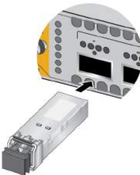
Figure 130. Installing 40Gbps Fiber Optic Transceivers in XEM2-4QS Line Cards
