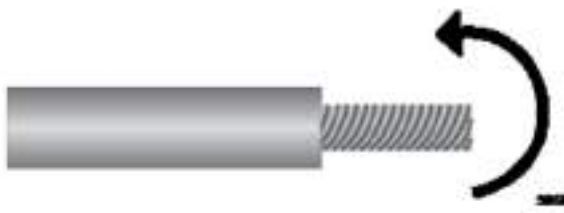
Figure 65. Wrapping the Wire Strands
