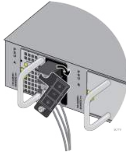
Figure 148. Accessing the Connecting Screws
