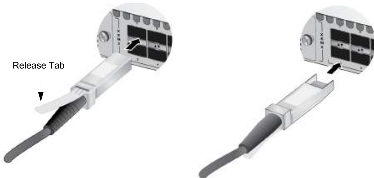
Figure 133. Installing SP10TW Direct Attach Cables
