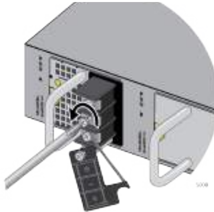
Figure 66. Loosening the Screw for the Negative (-)
