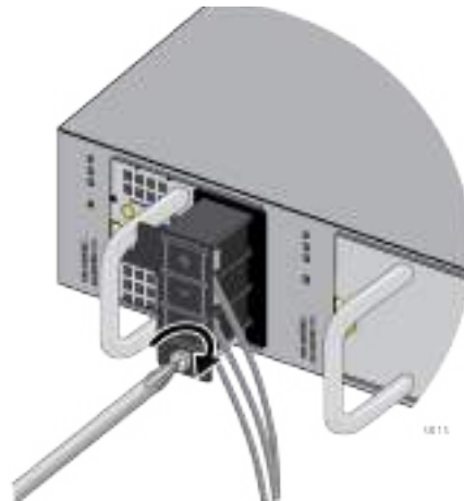
Figure 71. Tightening the Screw for the Cover Panel
