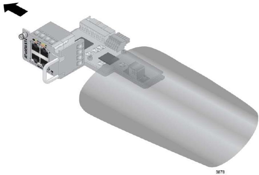
Figure 32. Removing the AT-x9EM/XT4 Card from the Anti-static Bag
