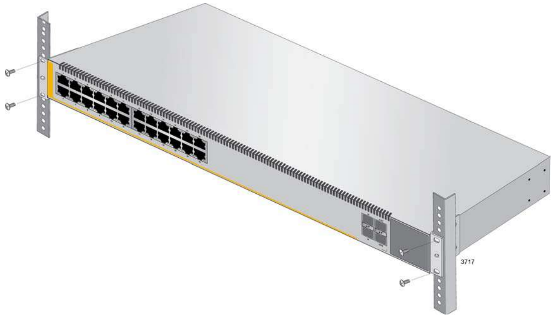
Figure 42. Installing the Switch in an Equipment Rack
