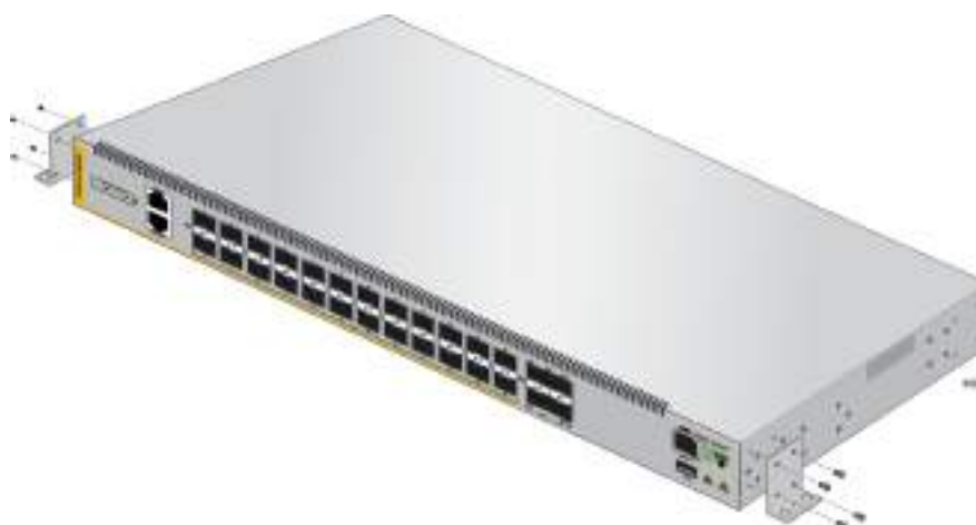
Figure 20. Attaching the Wall Mount Brackets
