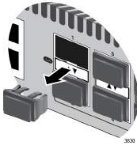
Figure 34. Removing the Dust Plug from a Transceiver Slot
