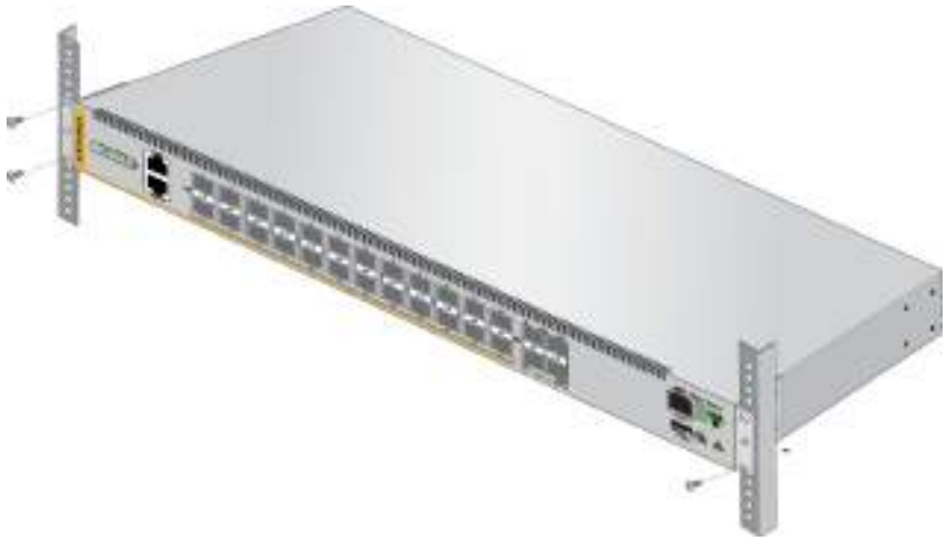
Figure 19. Mounting the Switch in an Equipment Rack
