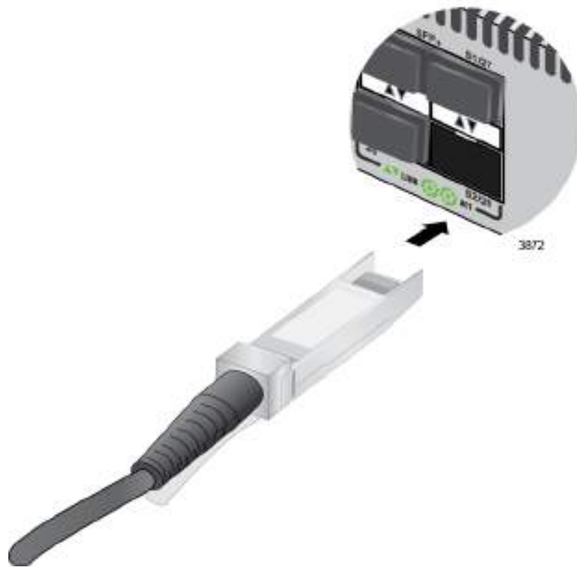
Figure 60. Installing a TwinAx Cable in Slot S2
