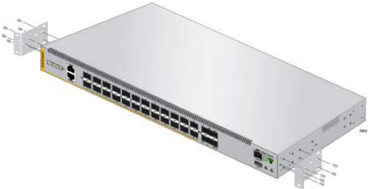
Figure 16. Attaching the Equipment Rack Brackets for a 19-Inch Rack, Front Mount
