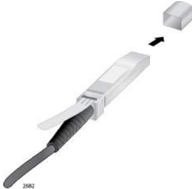
Figure 57. Removing the Dust Cover from a TwinAx Cable
