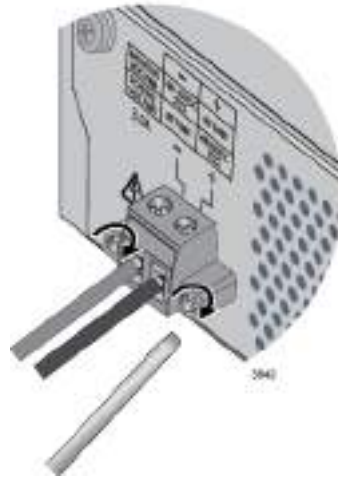
Figure 33. Securing the DC Connector to the Switch
