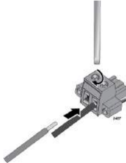
Figure 31. Inserting the Voltage and Return Wires
