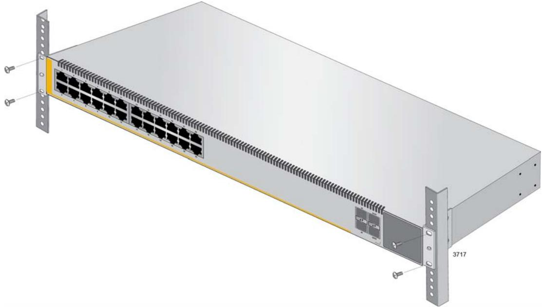
Figure 42. Installing the Switch in an Equipment Rack
