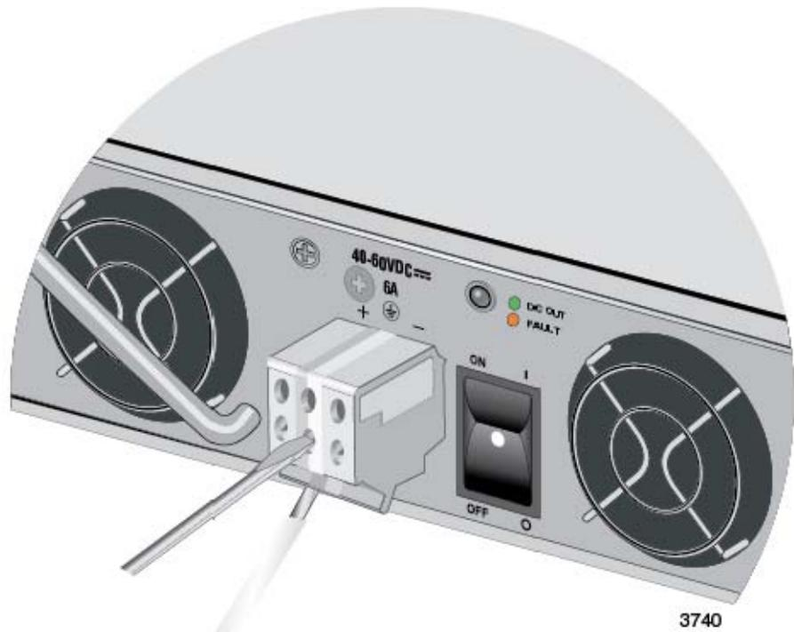
Figure 56. Connecting the Ground Wire to the DC Terminal Block
