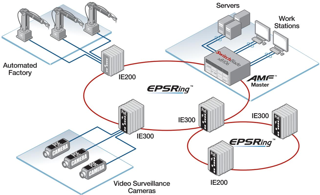
EPSRing™ ITU-T G.8032 provide high speed resilient ring connectivity; this diagram shows the IE Series in a double ring network topology.
