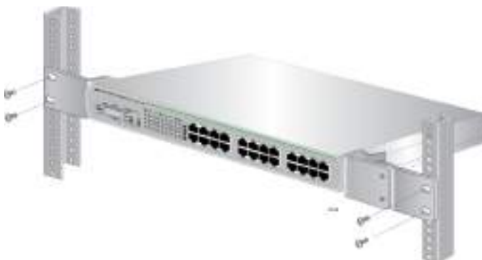
Figure 23. Attaching the Switch to an Equipment Rack
