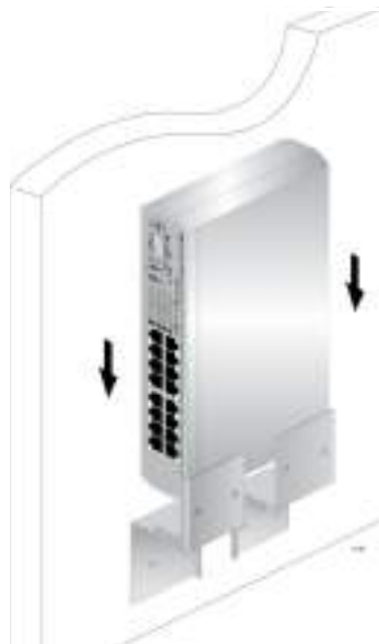
Figure 19. Placing the Switch into the Brackets
