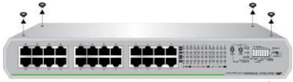
Figure 12. Removing Feet From the Chassis Bottom
