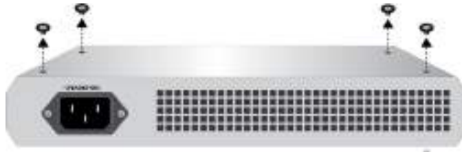
Figure 16. Removing the Rubber Feet
