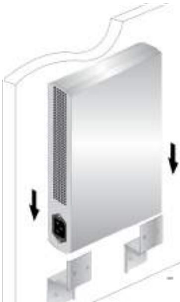
Figure 60. Placing the Switch into the Brackets
