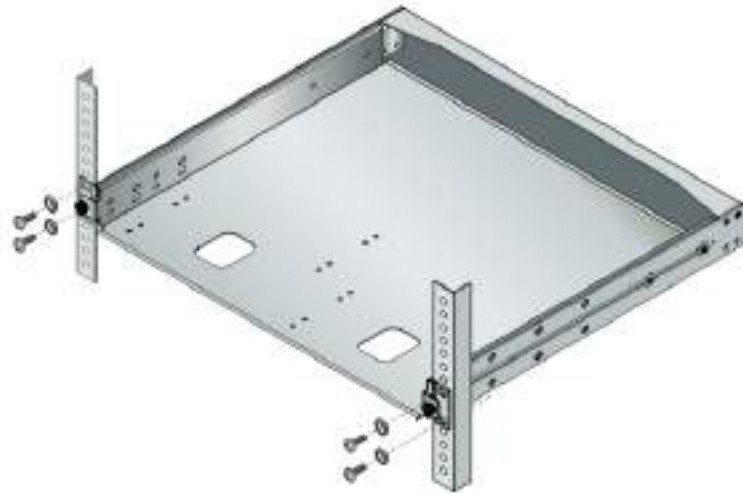
Figure 32. Installing the AT-RKMT-J15 Tray in a n Equipment Rack
