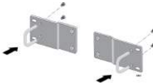
Figure 24. Attaching Handles to Brackets
