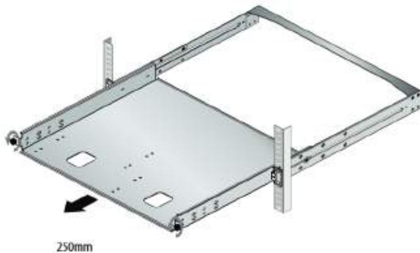
Figure 33. Pulling out the AT-RKMT-J15 Tray
