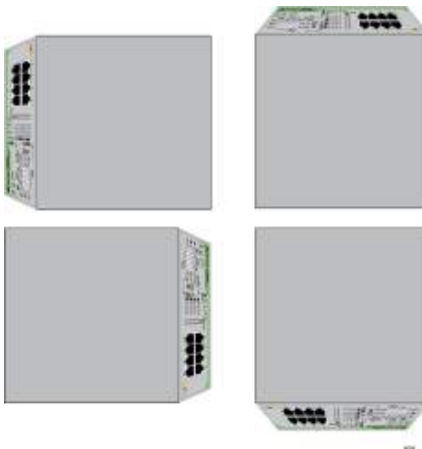
Figure 39. Orientations of the AT-GS920/8PS Switch on a Wall
