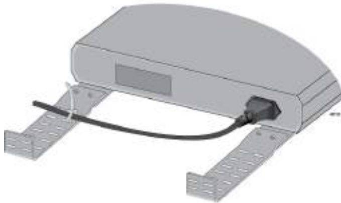
Figure 30. Securing the Power Cord Using Tie-wraps
