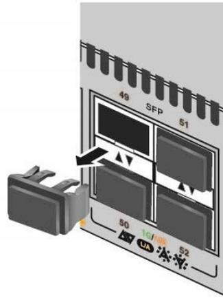
Figure 32. Removing the Dust Plug from an SFP Port
