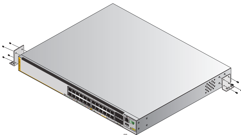
Figure 31. Installing Two Brackets on the AT-x530L-28GTX and AT-x530L-52GTX Switches
