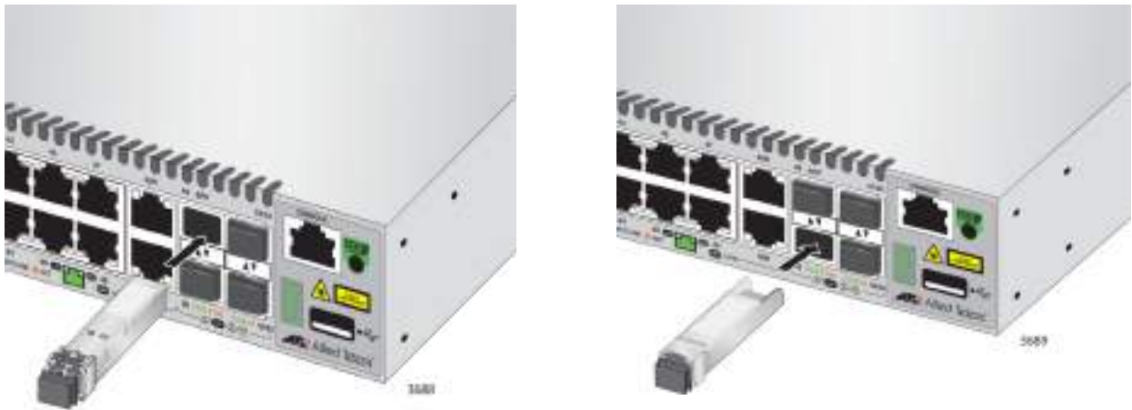
Figure 53. Installing an SFP Transceiver
