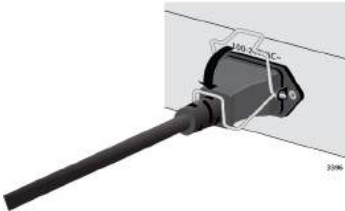
Figure 44. Lowering the Retaining Clip
