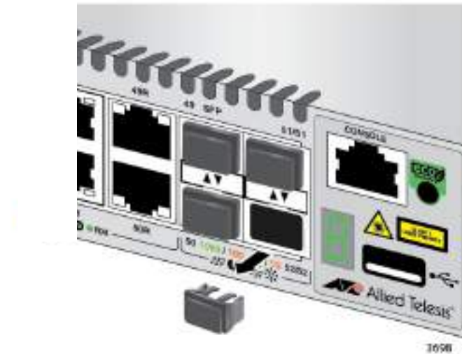
Figure 40. Removing the Dust Plug from the S2 Slot
