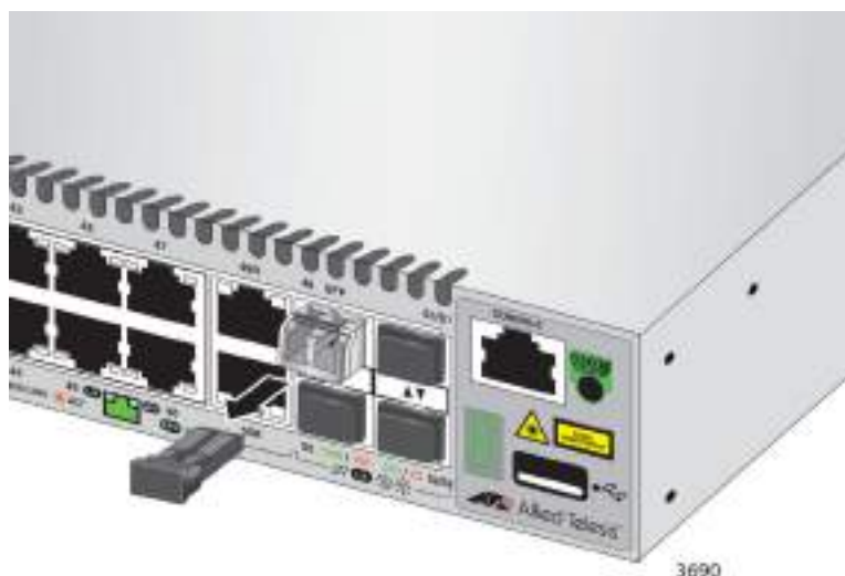
Figure 54. Removing the Dust Cover from an SFP Transceiver
