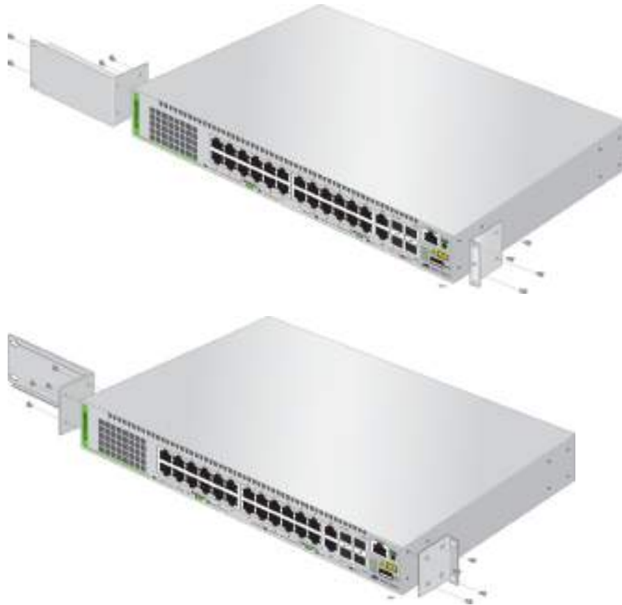
Figure 25. Installing Brackets on the AT-GS924MX Switch
