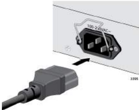
Figure 43. Plugging in the AC Power Cord
