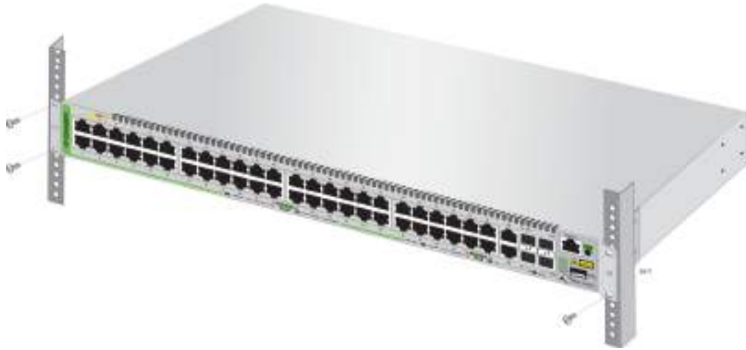
Figure 28. Mounting the Switch in an Equipment Rack
