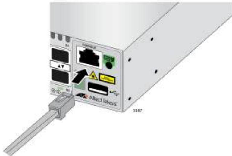
Figure 29. Connecting the Management Cable to the Console Port
