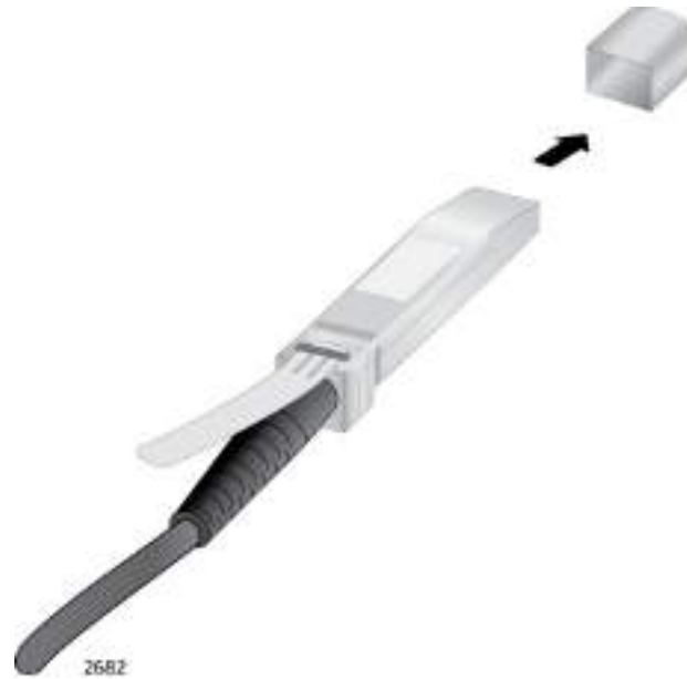
Figure 38. Removing the Dust Cover from the Transceiver
