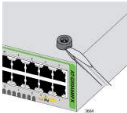
Figure 24. Removing the Rubber Feet
