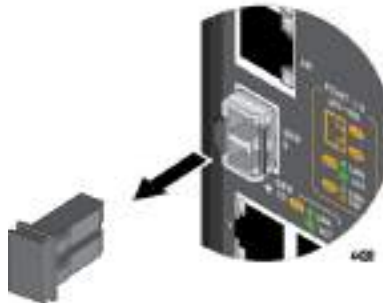
Figure 30. Remove Dust Cover from SFP Transceiver
