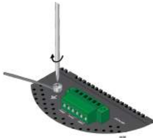
Figure 35. Secure Grounding Wire to the Switch
