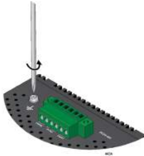
Figure 33. Loosen Grounding Screw
