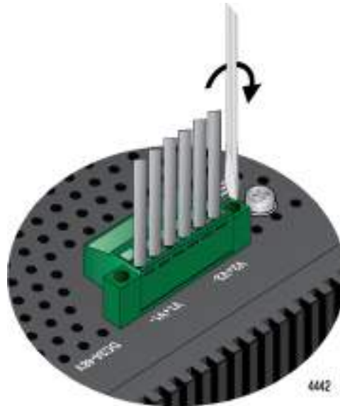
Figure 44. Fasten the Power/Alarm Connector to Chassis
