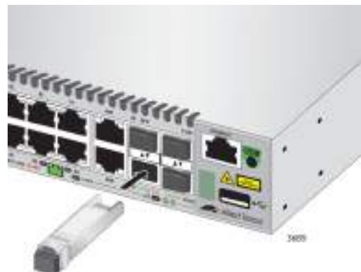
Figure 41. Installing an SFP Transceiver
