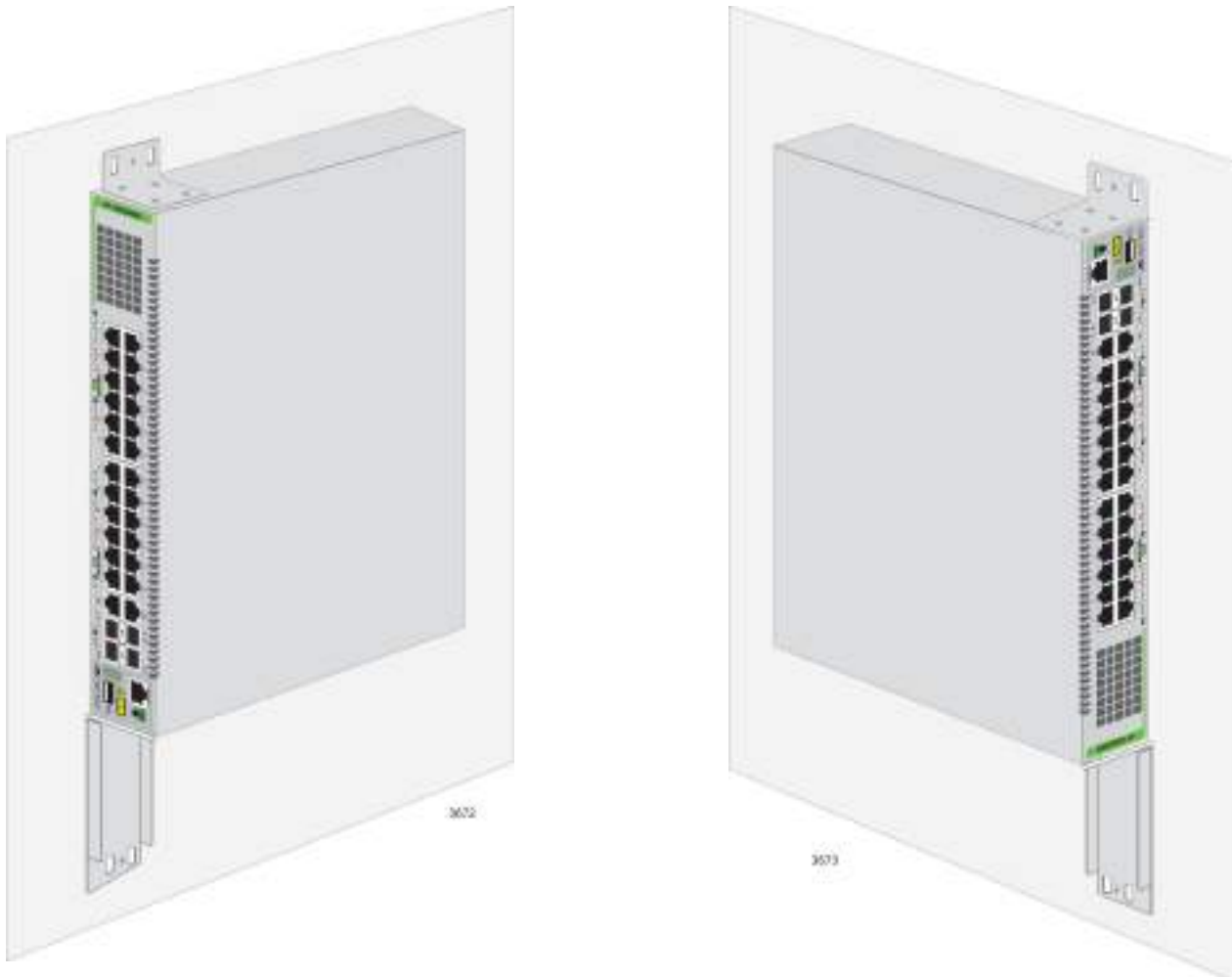
Figure 23. Positions of the AT-GS924MX Switch on a Wall
