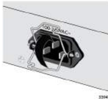
Figure 46. Raising the Retaining Clip
