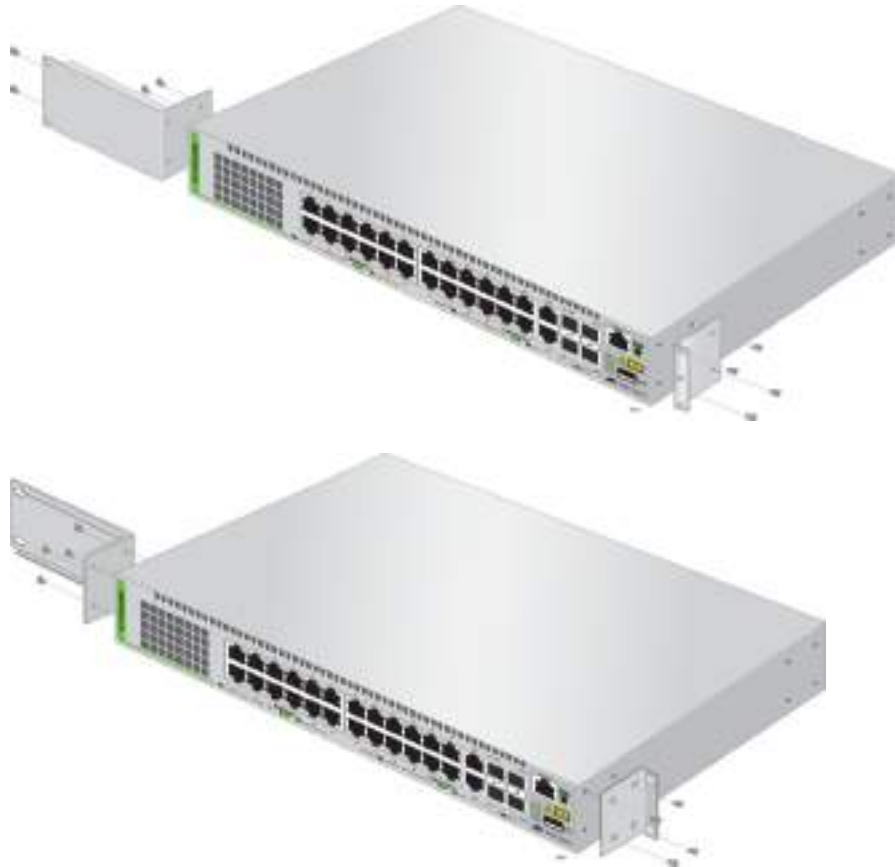
Figure 19. Installing Brackets on the AT-GS924MX Switch
