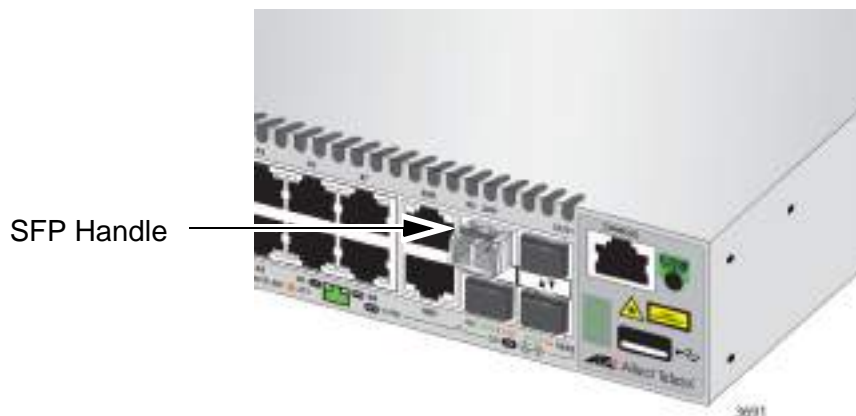
Figure 43. Positioning the SFP Handle in the Upright Position
