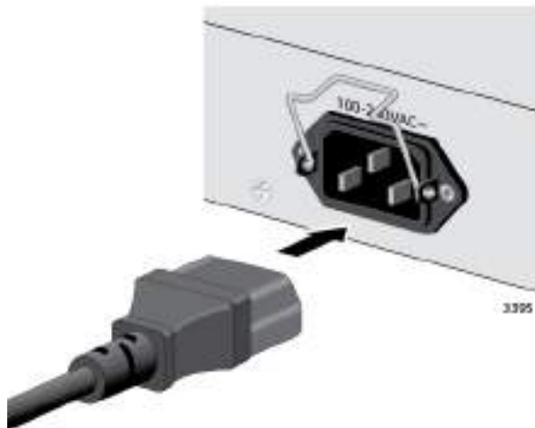
Figure 47. Plugging in the AC Power Cord
