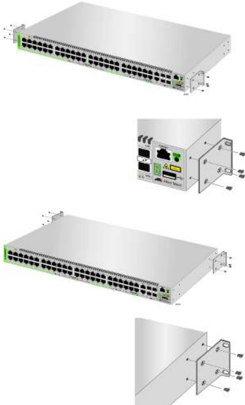
Figure 21. Attaching Brackets to the AT-GS924MX, AT-GS948MX, and AT-GS948MPX Switches (Continued)
