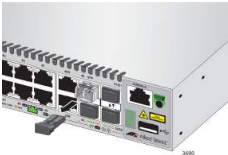
Figure 42. Removing the Dust Cover from an SFP Transceiver
