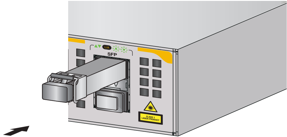
FIGURE 51. INSERTING AN SFP TRANSCEIVER INTO AN SFP SLOT
