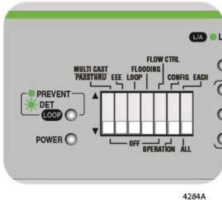
Figure 48. DIP Switch Settings for Disabling Loop Prevention
