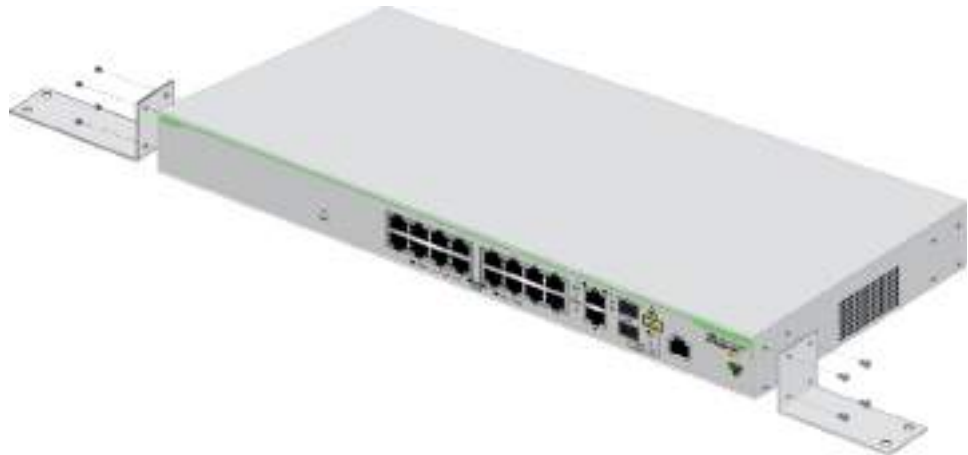
Figure 25. Attaching the Brackets to the Switch
