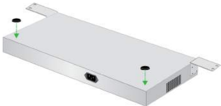
Figure 26. Attaching the Rubber Feet
