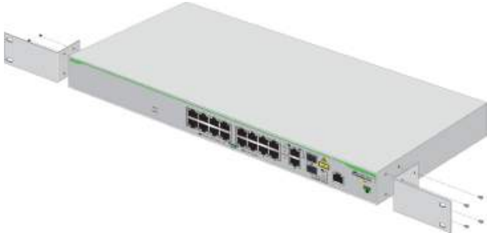
Figure 29. Attaching the Equipment Rack Brackets
