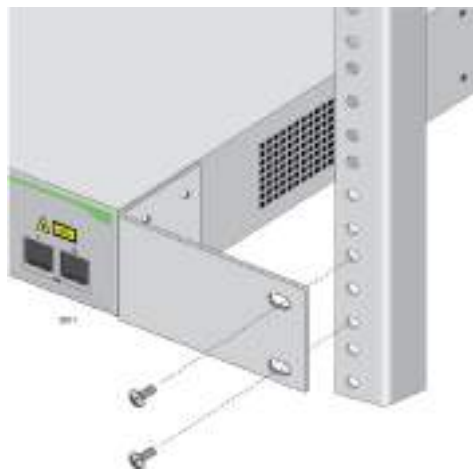
Figure 30. Mounting the Switch in an Equipment Rack
