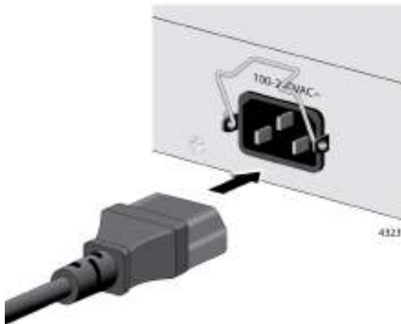
Figure 36. Plugging in the AC Power Cord
