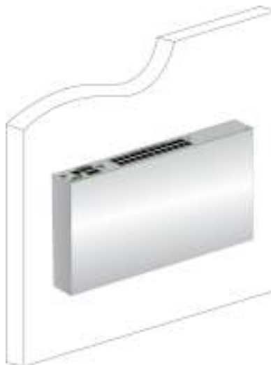
Figure 23. Correct Wall Installation
