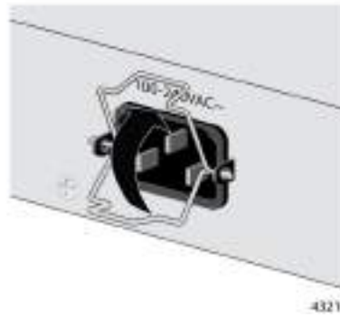
Figure 35. Raising the Retaining Clip
