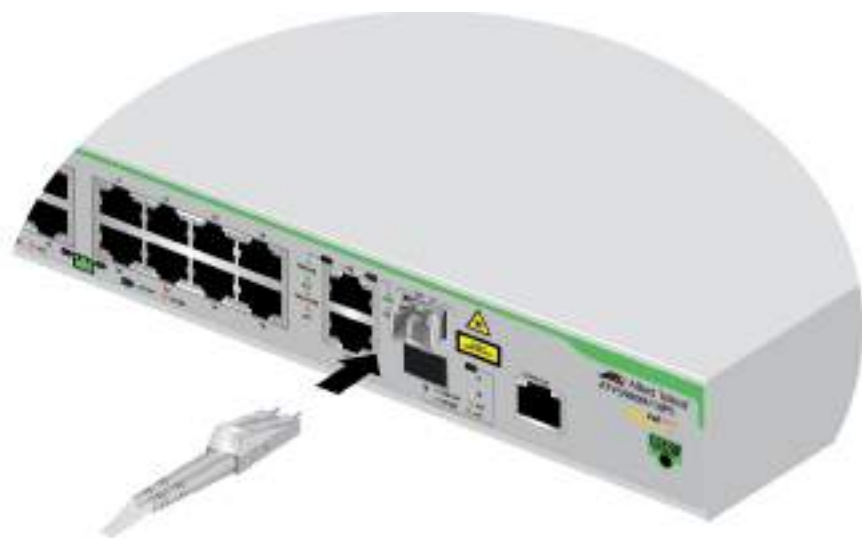
Figure 33. Connecting the Fiber Optic Cable to the SFP Module
