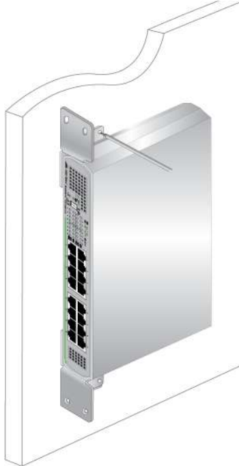
Figure 19. Marking the Screw Hole Locations
