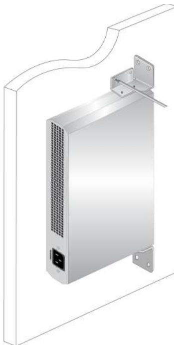
Figure 22. Marking the Screw Hole Locations
