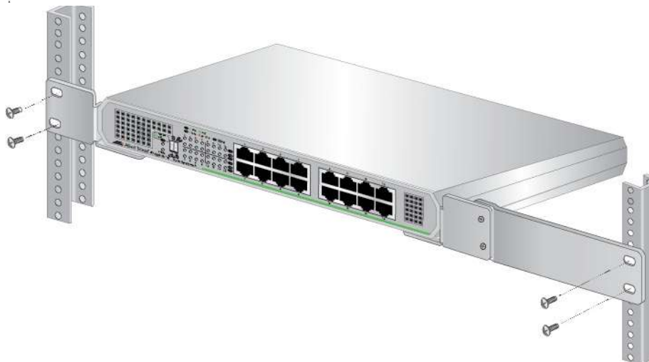
Figure 26. Attaching the Switch to an Equipment Rack
