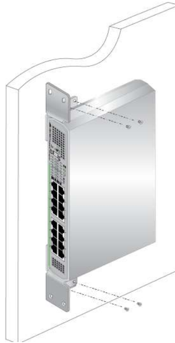
Figure 20. Driving the Screws through the Holes
