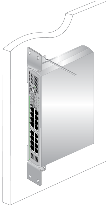
Figure 19. Marking the Screw Hole Locations
